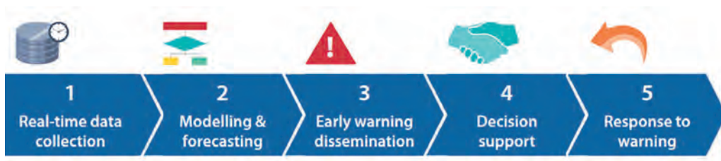
Figure 6. Main inter-related steps of the flood forecasting and warning system chain [26]
