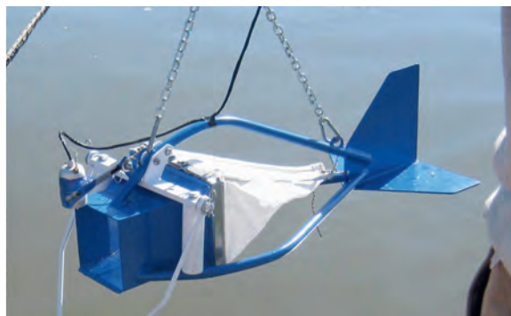
Figure 9. The Helley-Smith sampler with onboard camera mounted above the inlet (photo taken by the author)
