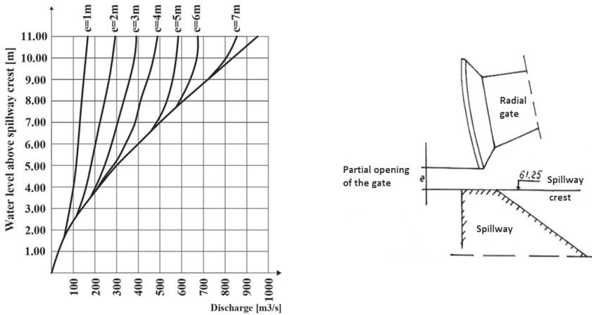
Figure 6. Rating curve for a radial gate [13]
