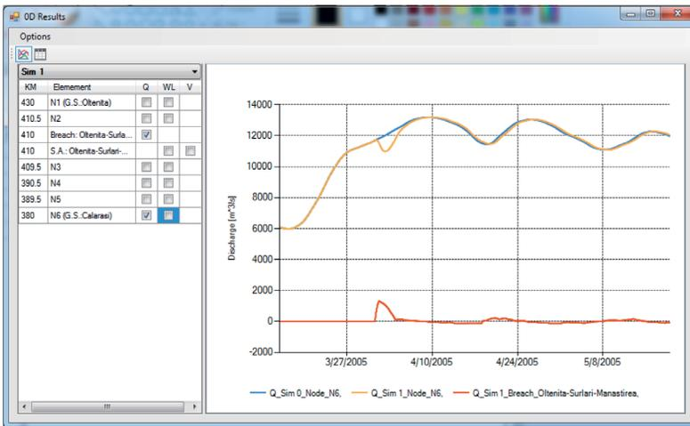
Figure 33. Hydraulic consequences of the Oltenița–Surlari–Mănăstirea enclosure flooding [6]
