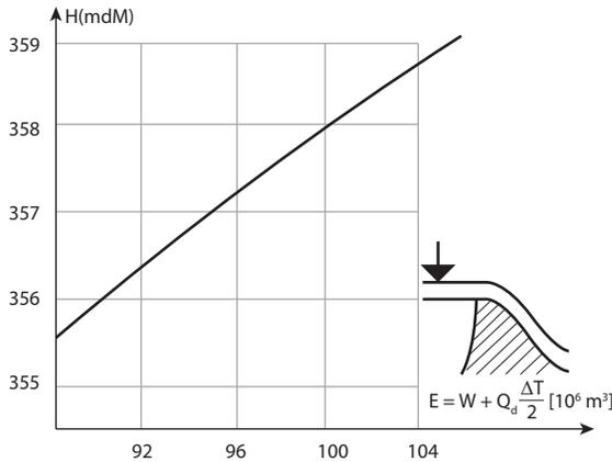
Figure 4. Elevation-outflow curve [11]
