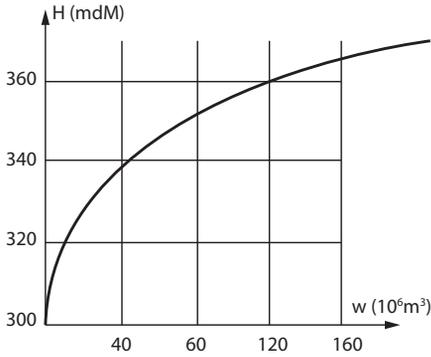
Figure 2. Elevation-storage curve [11]
