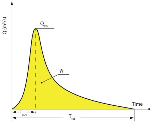
Figure 1. Parameters of the synthetic floods [5; 10]
