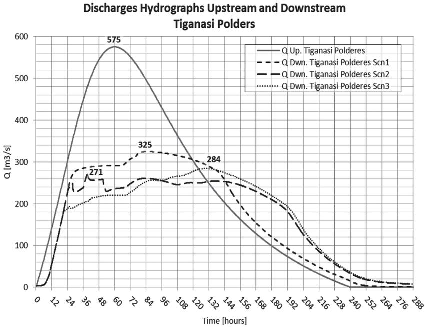
Figure 22. Discharge hydrographs upstream and downstream polders [8]
