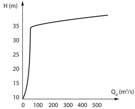
Figure 3. Elevation-outflow curve [11]
