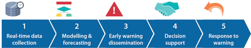
Figure 6. Main inter-related steps of the flood forecasting and warning system chain [26]
