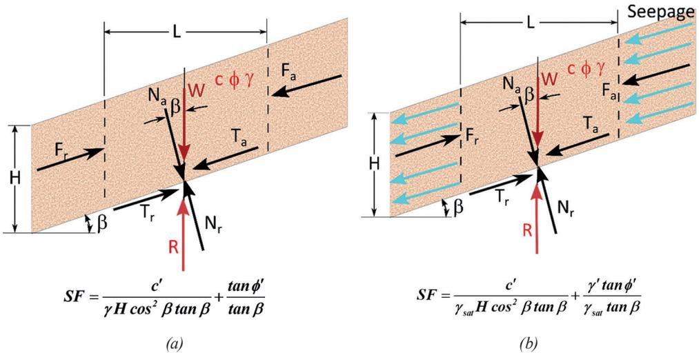
Figure 22. Infinite slope forces for (a) dry conditions and (b) seepage conditions (compiled by the author)
